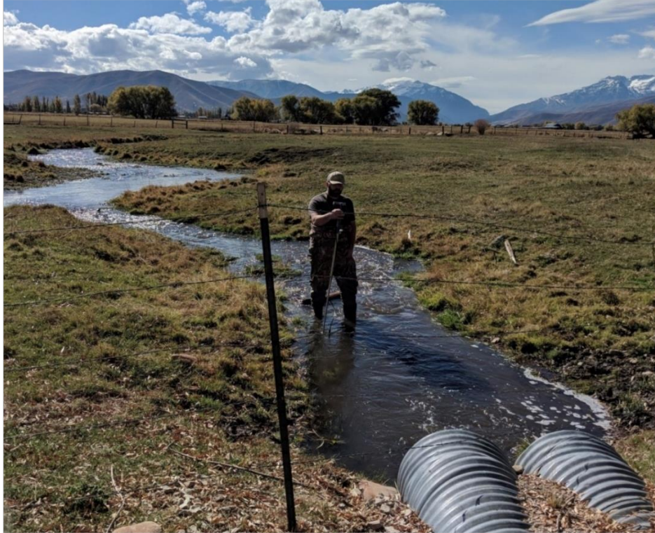
Figure 7. Collecting flow measurements in Spring Creek. Fall 2019.
